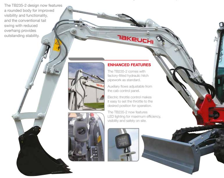
On site, the new 3.5 tonne TB235-2 mini excavator provides a compact size with familiar Takeuchi comfort and control.
