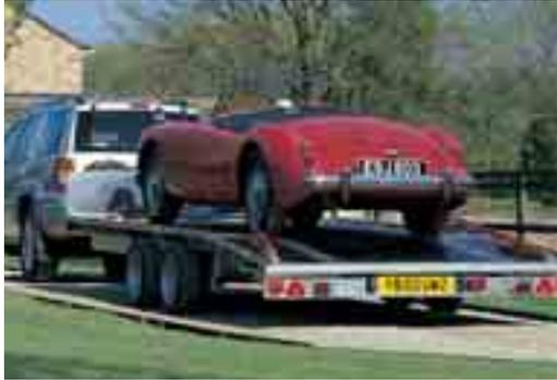
Closely related to the flatbed range, and with the addition of a sloping rear bed section, these trailers offer the flexibility of a flatbed with the added benefit of a low loading height to the rear of the trailer.
