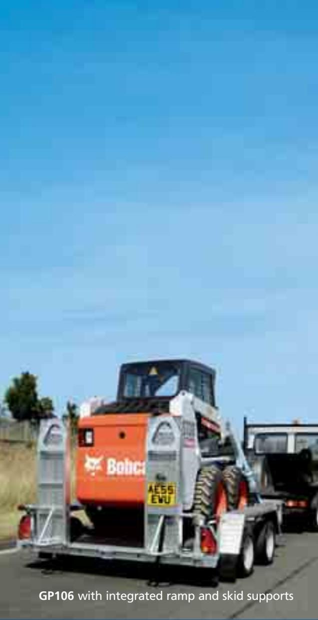
GP106 with integrated ramp and skid supports
